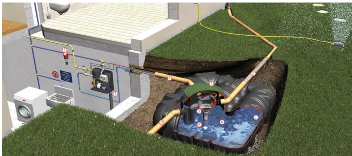
Image 3.2 Courtesy of Aquality – Underground Rainwater Storage tank. Source: GRAF, 2025.
