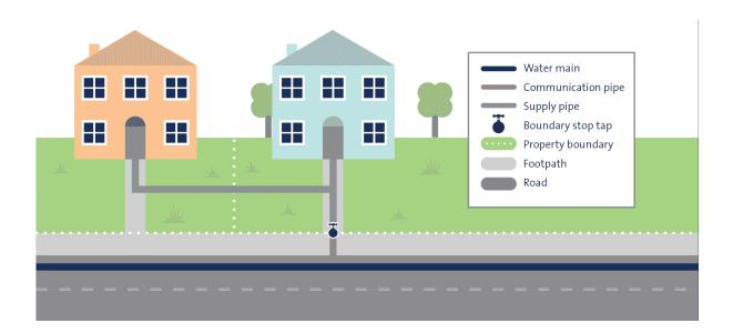
These are typical examples of a shared supply pipe layout:
