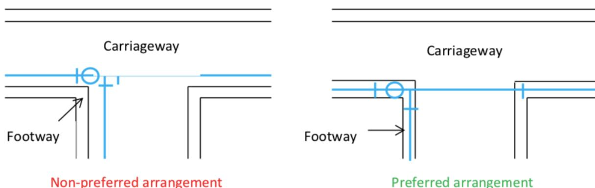
*If a change to road layout leads to fittings no longer being in the footway, liaison is suggested in order to move fittings or undertake mains diversion to maintain safe operation.*
