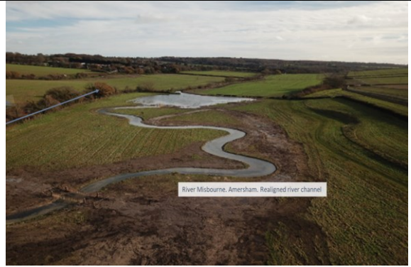
Figure 48: Amersham to Quarrendon Mill 2020 post-river restoration (channel realignment)
